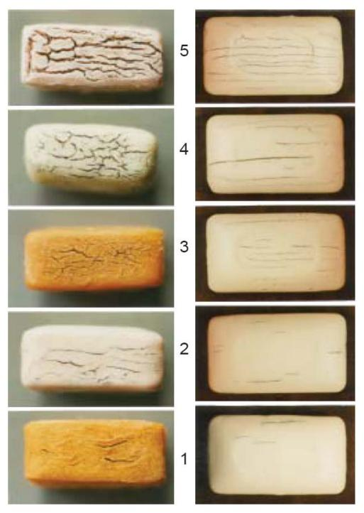
End cracking scale
